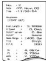
Record printout Automatic/manual data printout on high-resolution thermprinter
